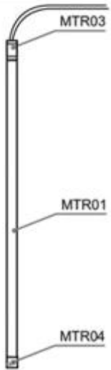
Step 1 Connect the MTR03 and MTR04 to the MTR01
